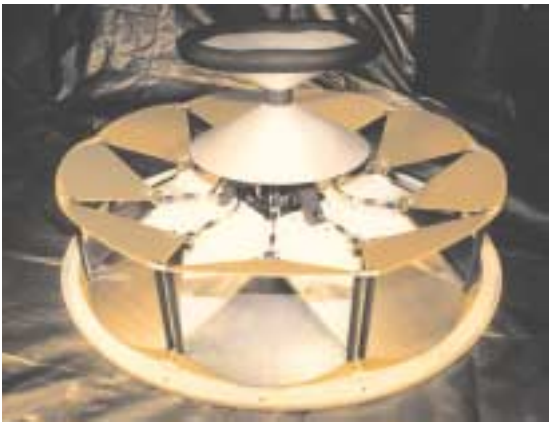
641M Antenna Elements (Radome Removed)
