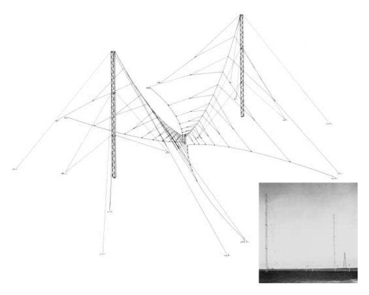
The quality of short range shortwave broadcasting can be greatly enhanced with a properly chosen antenna. Ideally, the antenna should handle high power to insure high signal-to-noise ratio at the receiver, have a wide frequency bandwidth for selection of the appropriate frequency, allow diplexing of two transmitters on one antenna, and produce radiation at high elevation angles.
