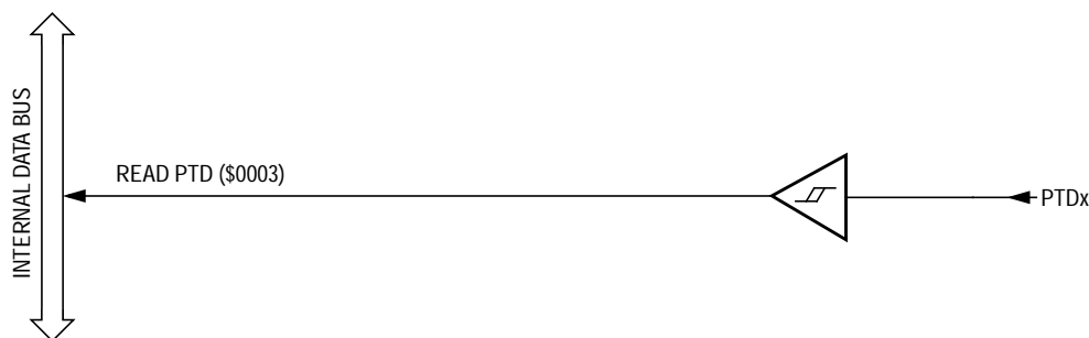
Figure 15-12. Port D Input Circuit
