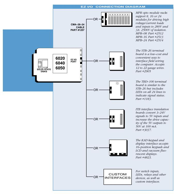
The EZ I/O port has 24 digital lines that are individually programmable as either 5V inputs or outputs. They will sink and source 15 mA. The lines have pull—up/pull—down resistors for convenient interfacing to a variety of external devices. The port is supported with both BIOS calls and CAMBASIC. The 6020 has two EZ I/O ports.
