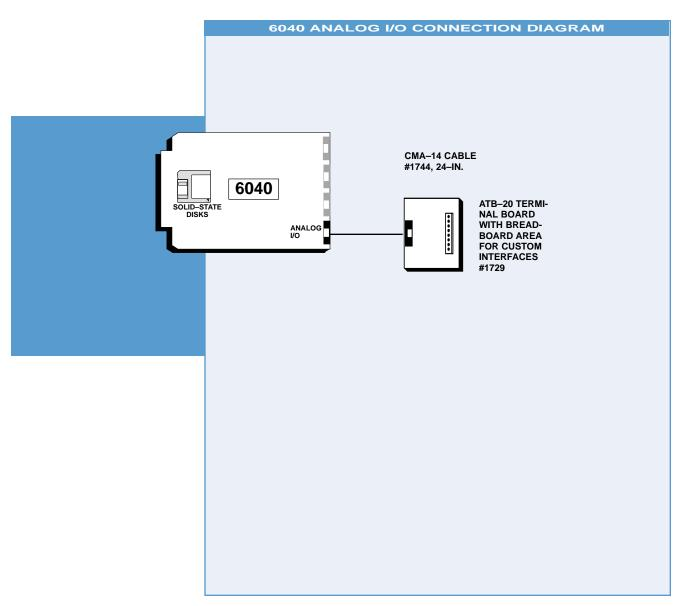
Analog I/O: The 6040 has eight, 12-bit analog inputs with software programmable ranges. The two analog voltage outputs have jumper programmable ranges.
