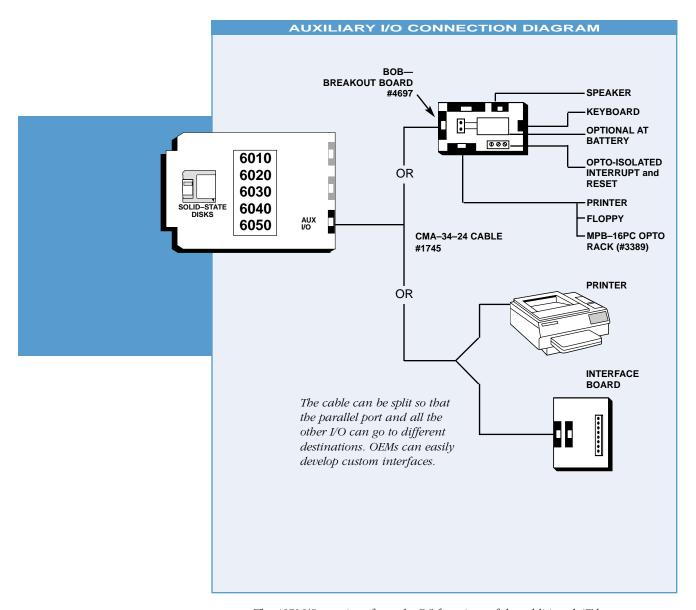
The AUX I/O port interfaces the PC functions of the additional AT battery, keyboard, parallel port, speaker port and opto-isolated interrupt inputs. This clustering of functions saves card space, reduces the number of cables, and makes it easy for the OEM to develop low-cost, custom interfaces. The AT battery operates in parallel with the on-card battery to extend battery life. The 6010 has floppy and hard disk ports on-card.
