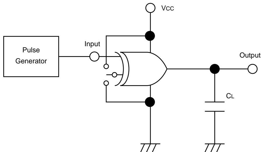
Note: open output when measuring supply current
