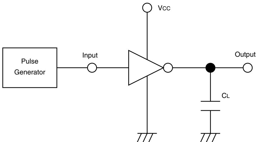
Note: open output when measuring supply current
