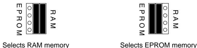
If you set the memory to RAM, you can download programs and set break-points in memory with the command monitor. With a read-only EPROM selected and installed, you can't perform these operations. In addition, you must include the section of code listed below in the EPROM if you want to use the single-step and run capabilities from the command monitor.
