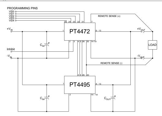
Input Capacitors: Although not necessary for stable operation, Cin will reduce input ripple. Cin = 33µF is suggested.
