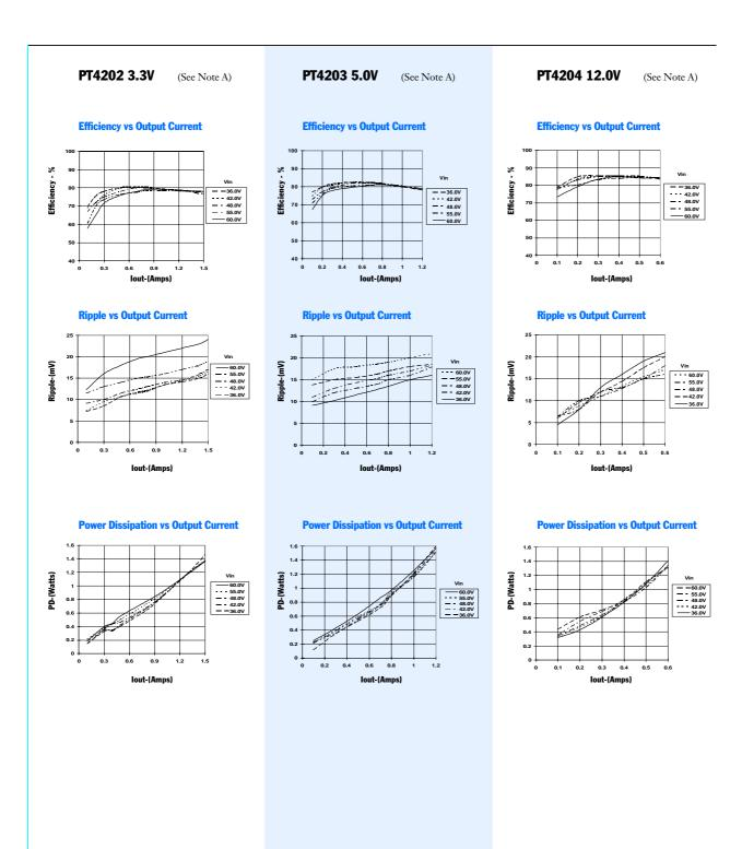
Note A: All data listed in the above graphs, except for derating data, has been developed from actual products tested at 25°C. This data is considered typical data for the DC-DC Converter.
