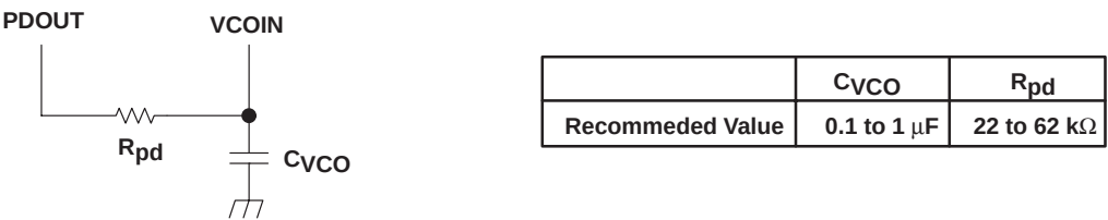
Figure 8. Resistor and Capacitor Connection
