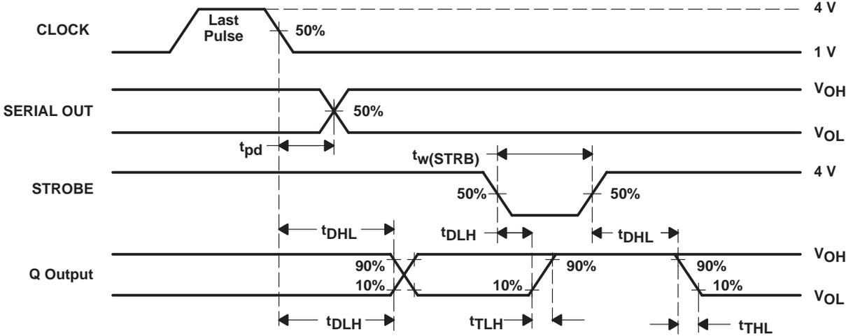
Figure 2. Switching Characteristics
