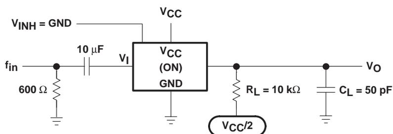
Figure 10. Sine-Wave Distortion
