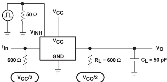
Figure 8. Crosstalk Between Control Input and Switch Output
