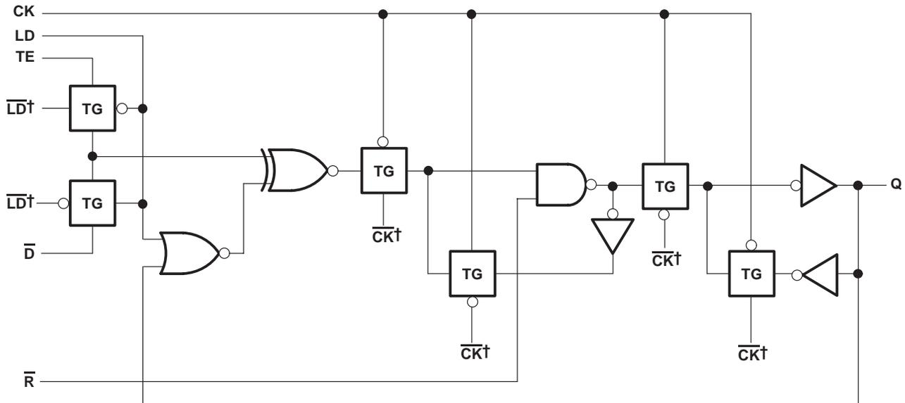
† The origins of  $\overline{LD}$  and  $\overline{CK}$  are shown in the logic diagram of the overall device.
