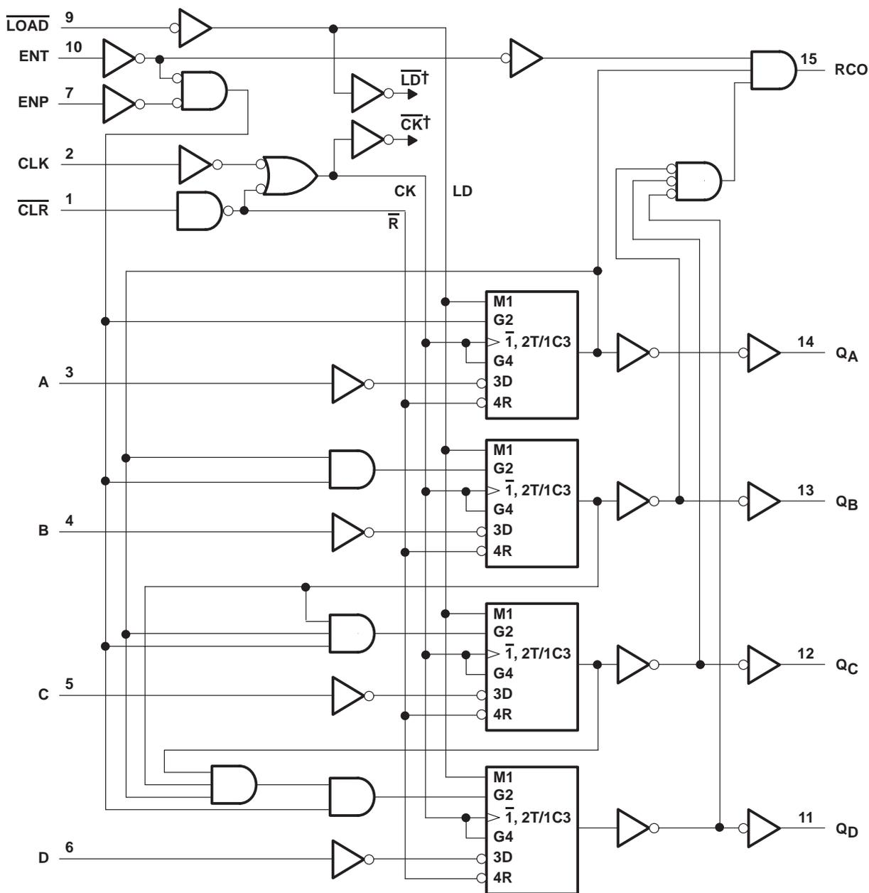
† For simplicity, routing of complementary signals  $\overline{\text{LD}}$  and  $\overline{\text{CK}}$  is not shown on this overall logic diagram. The uses of these signals are shown on the logic diagram of the D/T flip-flops.
