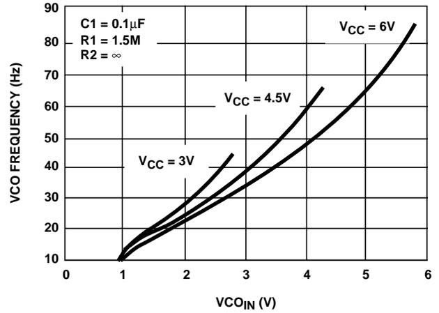
FIGURE 19. HC7046A TYPICAL VCO FREQUENCY vs VCO<sub>IN</sub> (R1 = 1.5MΩ, C1 = 0.1µF)
