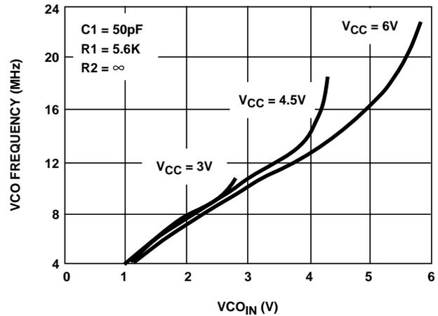
FIGURE 23. HC7046A TYPICAL VCO FREQUENCY vs VCO<sub>IN</sub> (R1 = 5.6kΩ, C1 = 50pF)
