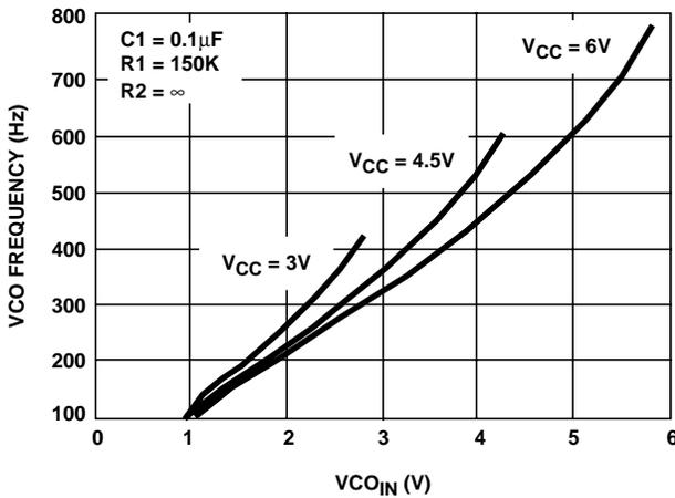
FIGURE 20. HC7046A TYPICAL VCO FREQUENCY vs VCO<sub>IN</sub> (R1 = 150kΩ, C1 = 0.1µF)
