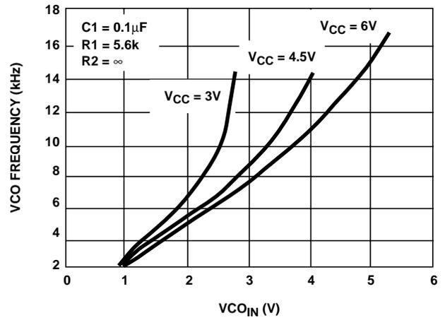
FIGURE 21. HC7046A TYPICAL VCO FREQUENCY vs VCO<sub>IN</sub> (R1 = 5.6kΩ, C1 = 0.1µF)
