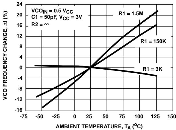
FIGURE 24. HC7046A TYPICAL CHANGE IN VCO FREQUENCY vs AMBIENT TEMPERATURE AS A FUNCTION OF R1 (V<sub>CC</sub> = 3V)
