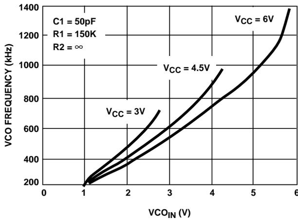
FIGURE 22. HC7046A TYPICAL VCO FREQUENCY vs VCO<sub>IN</sub> (R1 = 150kΩ, C1 = 0.1μF)
