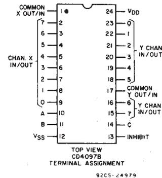
\*When these devices are used as demultiplexers, the channel in/out terminals are the outputs and the common out/in terminals are the inputs.
