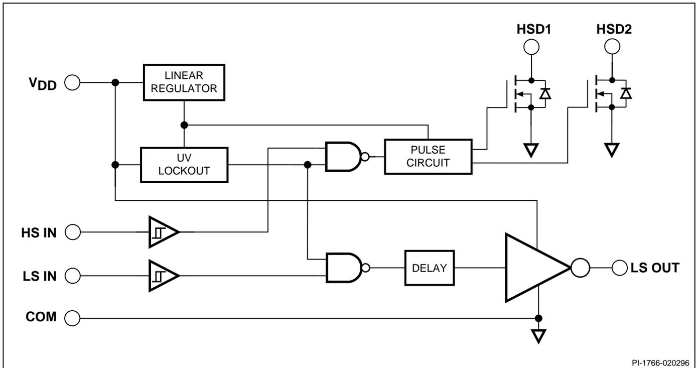
Figure 3. Functional Block Diagram of the INT202
