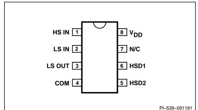
Figure 2. Pin Configuration.
