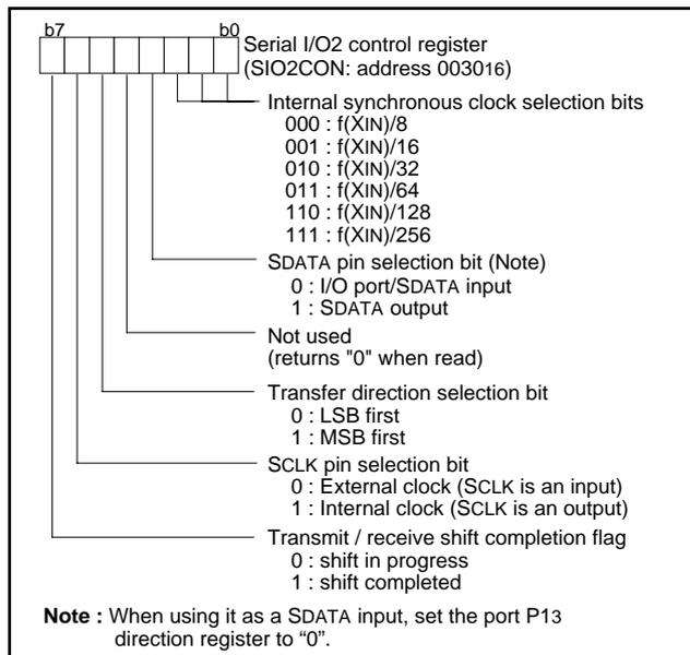
Fig. 29 Structure of serial I/O2 control registers
