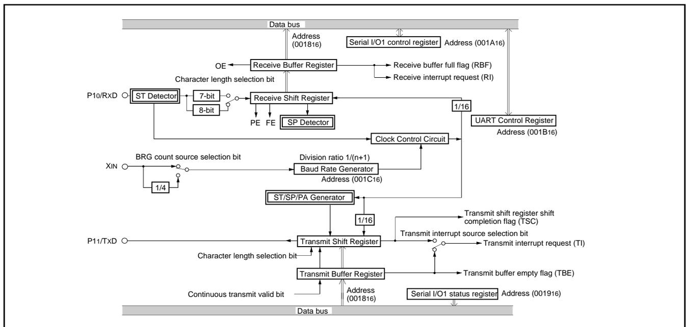
**Fig. 19 Block diagram of UART serial I/O**
