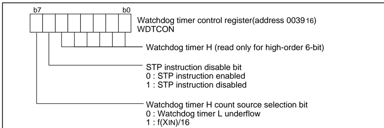
Fig. 36 Structure of watchdog timer control register
