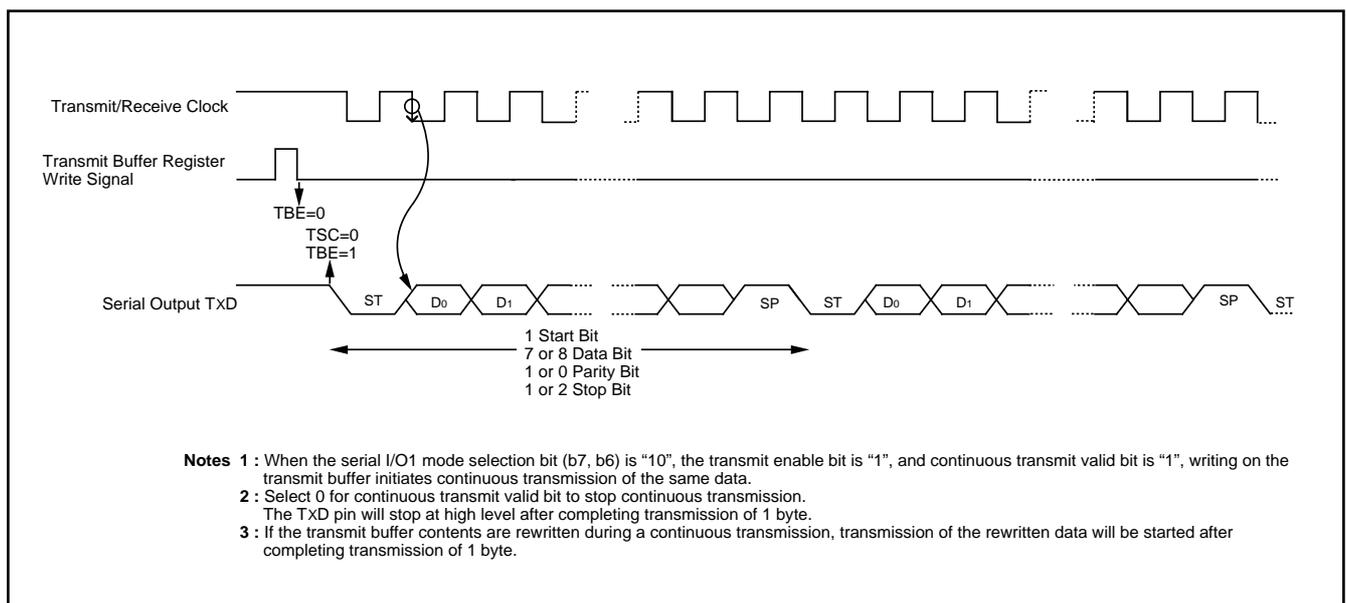
Fig. 21 Continuous transmission operation of UART serial I/O
