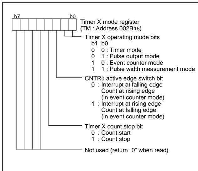
Fig. 16 Structure of timer X mode register
