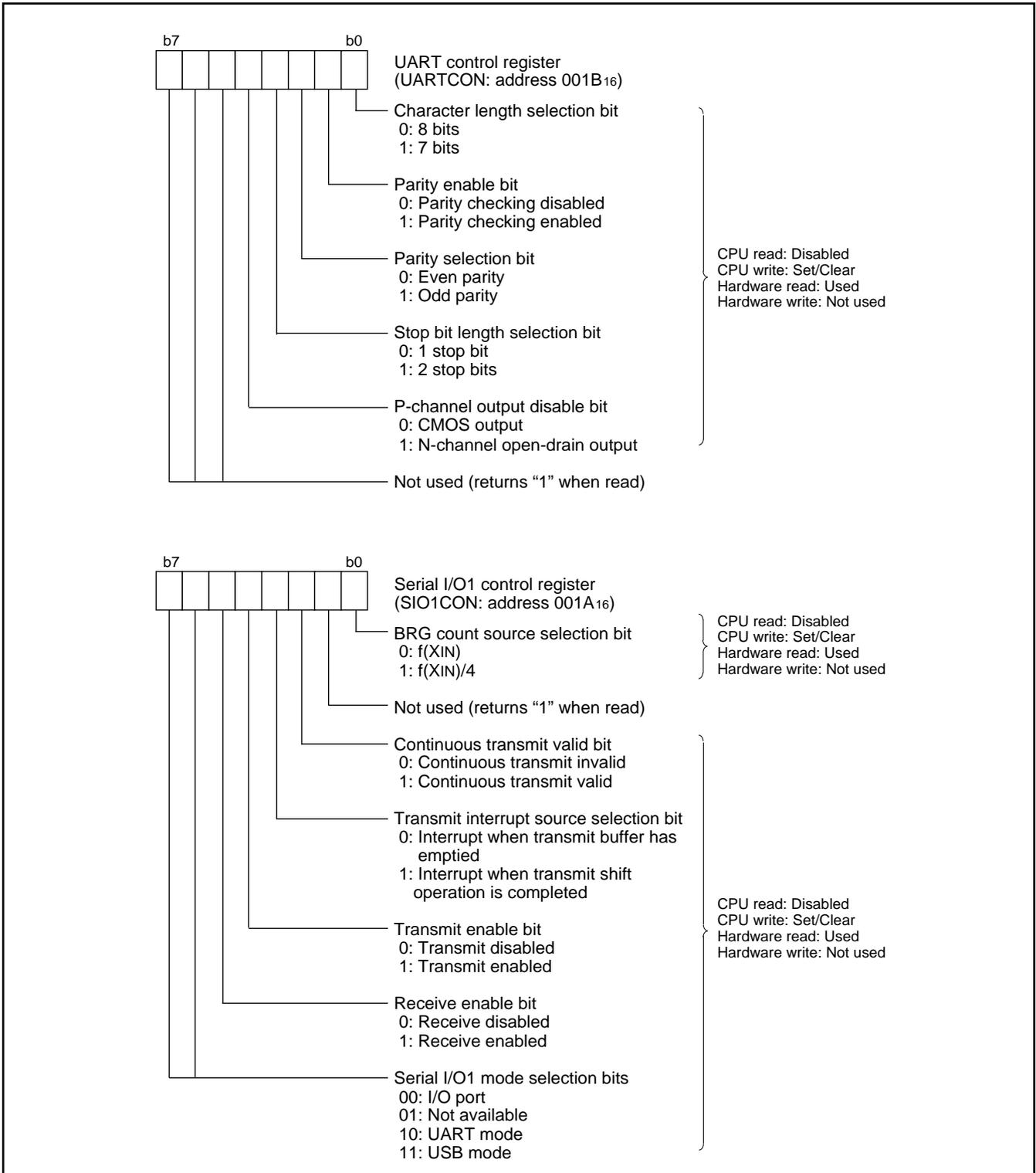
Fig. 28 Structure of serial I/O1-related registers (5)
