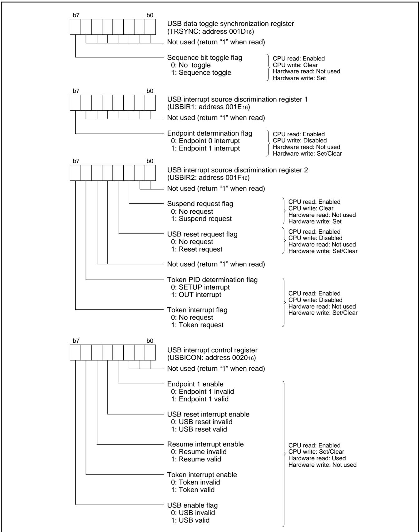
Fig. 25 Structure of serial I/O1-related registers (2)
