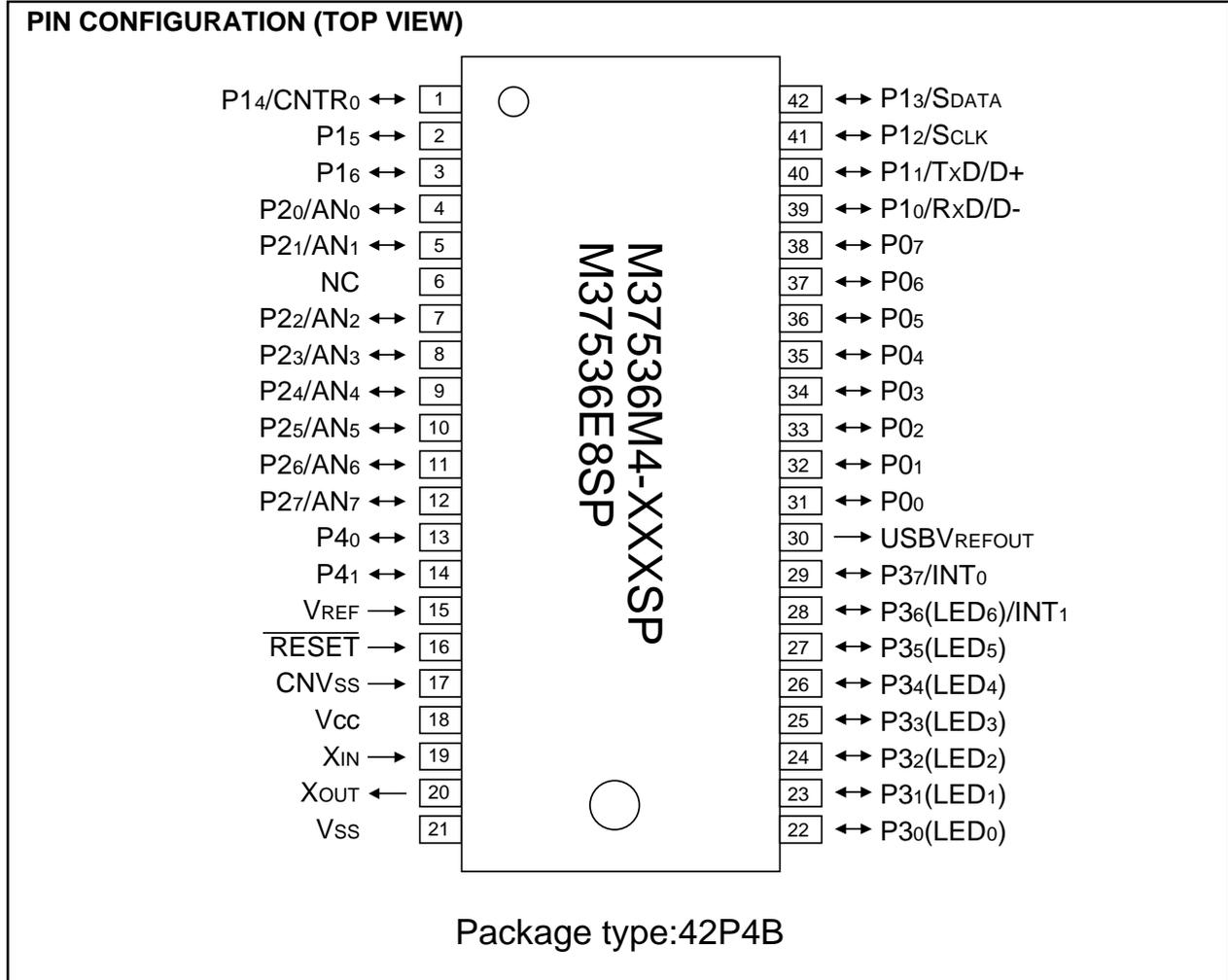
Fig. 1 Pin configuration of M37536M4-XXXSP, M37536E8SP
