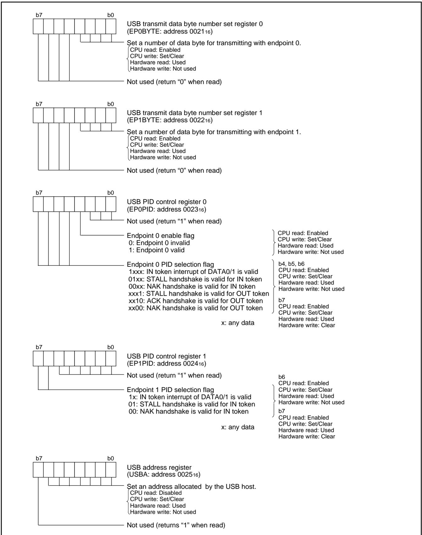
Fig. 26 Structure of serial I/O1-related registers (3)
