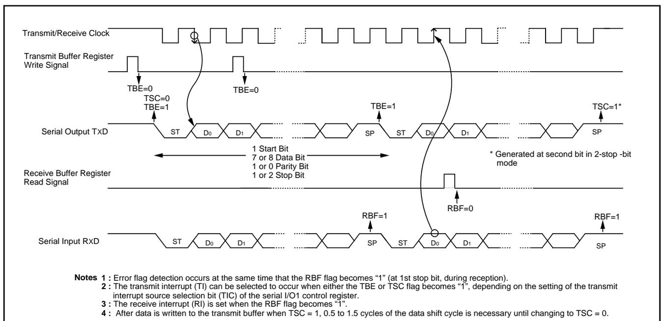
**Fig. 20 Operation of UART serial I/O function**
