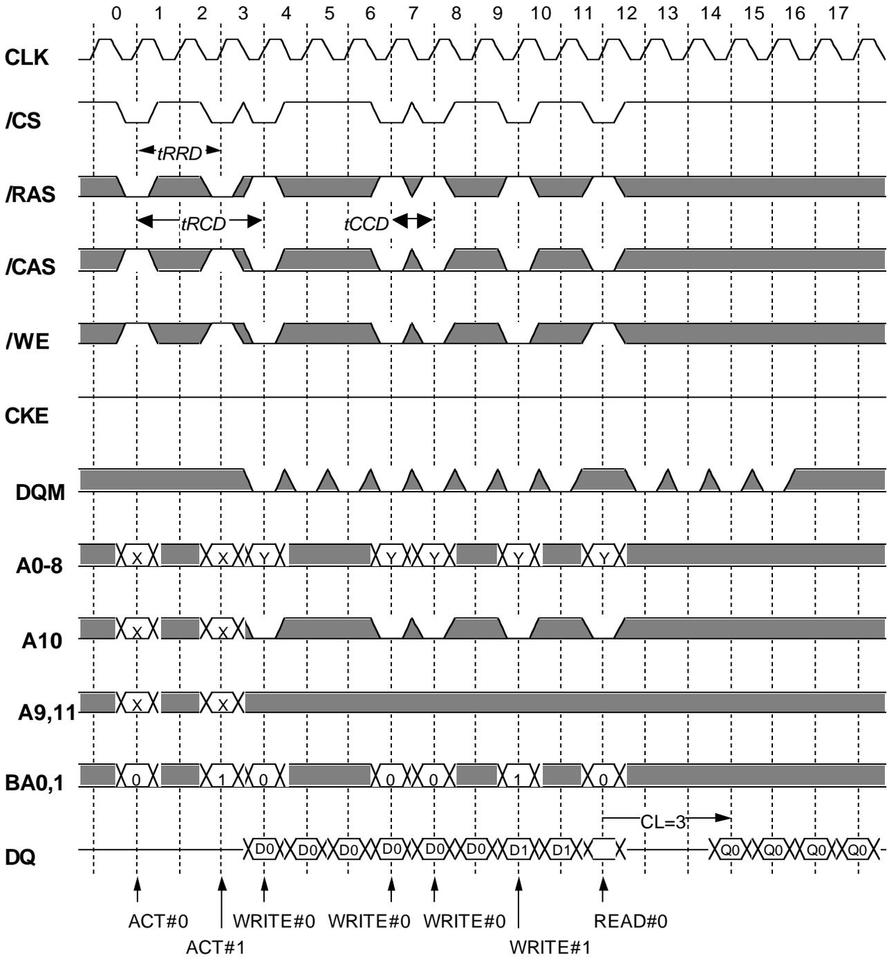
Burst Write can be interrupted by Write or Read of any active bank.
