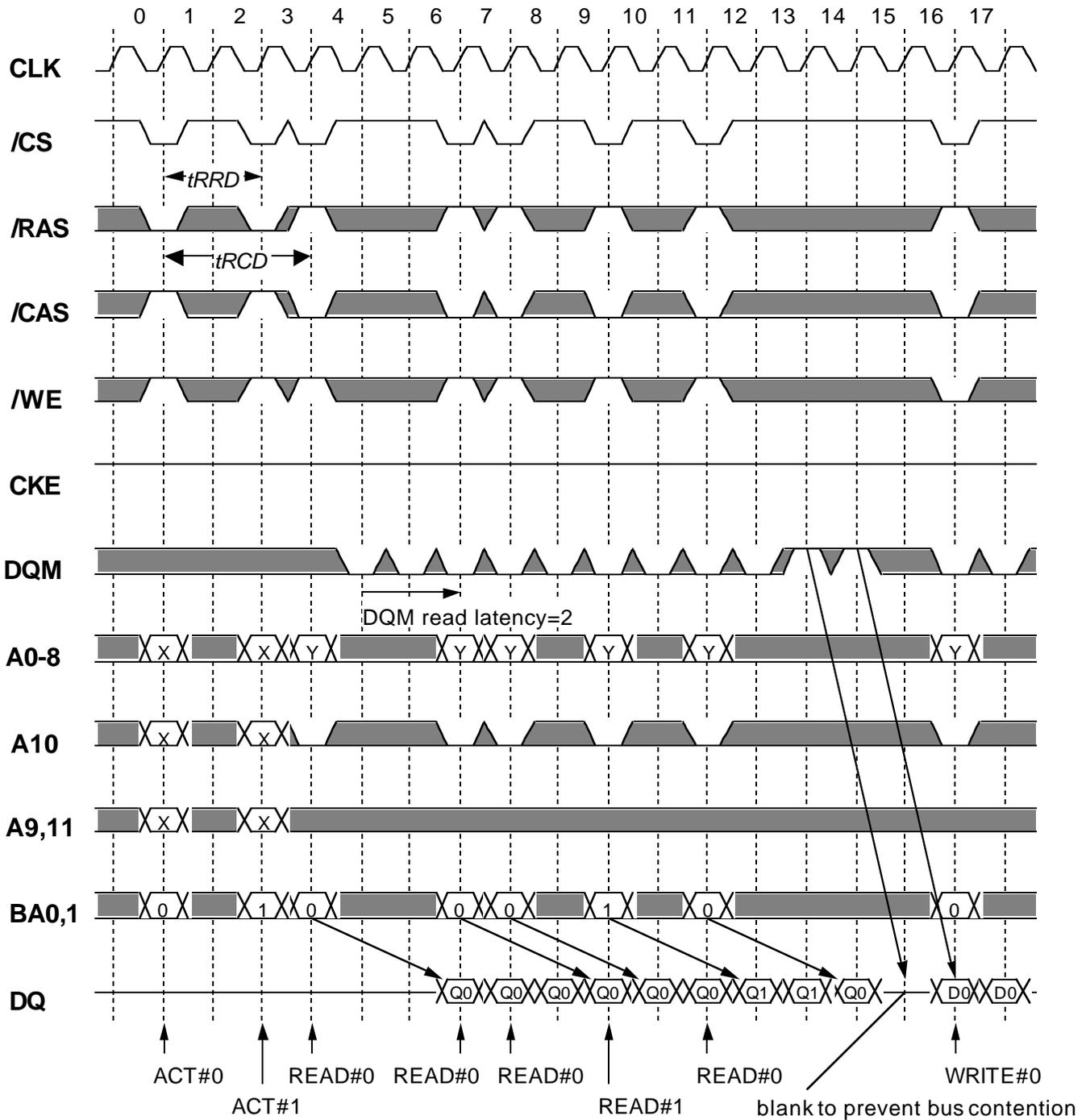
Burst Read can be interrupted by Read or Write of any active bank.
