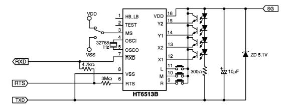
The  $\overline{\mathsf{RXD}}$  pin is NMOS open drain output.
