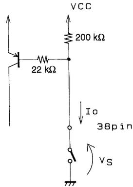
The power switch is on when the power switch pin is connected to ground.
