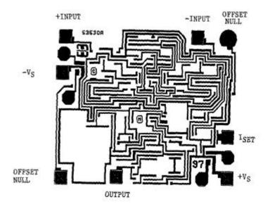
Die bonding pad locations and electrical functions
