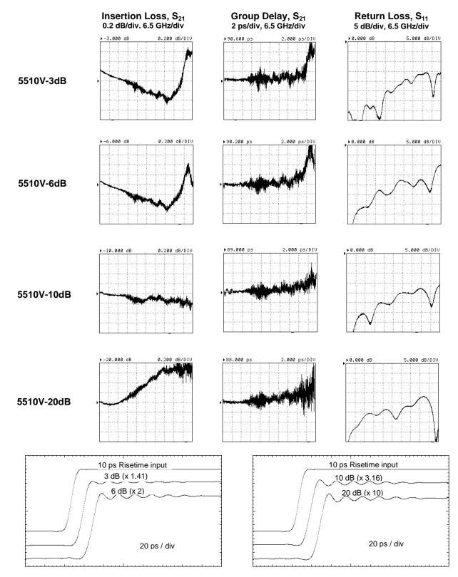
**Notes:** All plots are from randomly selected samples. The 10 ps step responses were measured using a PSPL Model 4015C pulse generator and an HP-54750, 50 GHz oscilloscope. The frequency responses were measured using an Anritsu 37397A, 65 GHz vector network analyzer.
