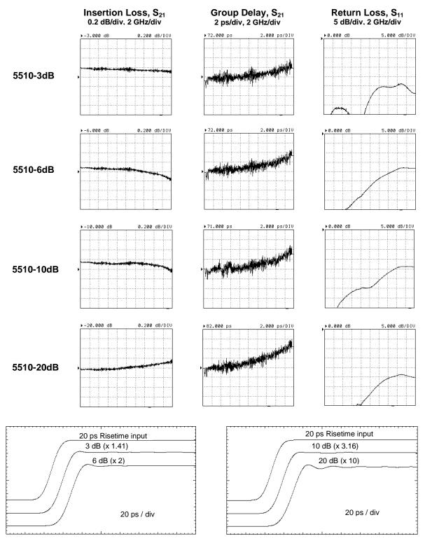
**Notes:** All plots are from randomly selected samples. The 20 ps step responses were measured using a PSPL Model 4015C pulse generator and an HP-54750, 50 GHz oscilloscope. The frequency responses were measured using an Anritsu 37397A, 65 GHz vector network analyzer.
