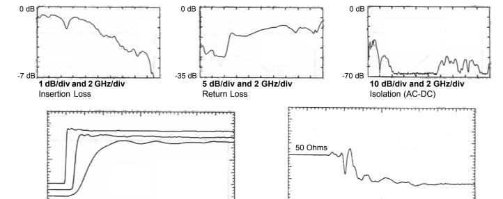
20%/div. Top to bottom: 500 ps/div, 100 ps/div and 20 ps/div 10 ps Step Response
