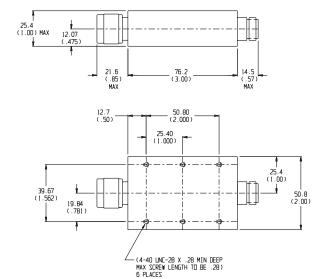
NOTE: All dimensions are given in mm (inches) and tolerances are .X±0.5 (0.02) & .XX+0.25 (0.01), unless otherwise specified.
