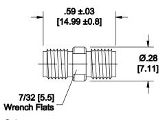
Note: Dimensions in Brackets are Expressed in Millimeters and are for Reference Only. Selected units featuring very low return loss (VSWR) and/or optimized RF leakage are also available.
