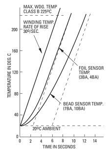
Example of sensor temperature tracking capability with locked rotor conditions.
