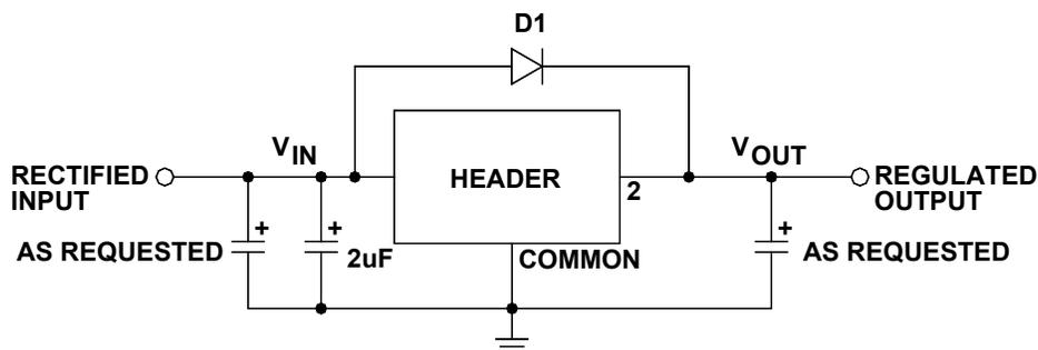
**Note:** D1 should be installed for input safety.
