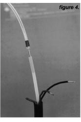
The desiccant changes from blue to red as it's drying capacity becomes diminished. The Vent Filter/Vapor Trap can be exposed to air, industrial gases, refrigerants, organic liquids and solvents. It should not be used when ammonia is present.
