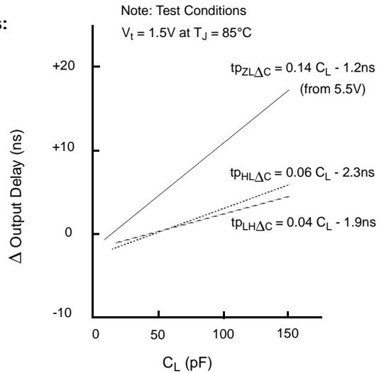
Output Propagation Delay Derating vs Output Voltage Level
