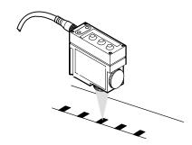
The Photoswitch Type 42CRC Series 4000 LED Color Registration Mark Control with Automatic Gain Control (AGC) is a fixed focus diffuse-reflective scanning device designed to detect preprinted registration marks against contrasting backgrounds. Detection of the marks is achieved by sensing the difference in the gray-scale response to the mark and background.
