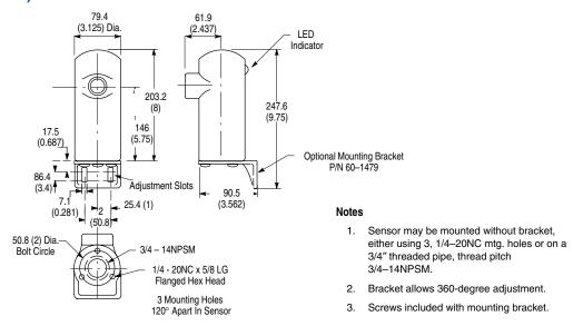
Note: Do not use lockwashers with supplied whiz-lock mounting screws.
