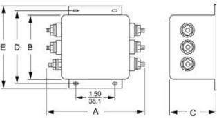
Mounting slots:  $\frac{.250 \times .156}{6.35 \times 3.96}$ Torque 27  $\pm$  3 in.lb. Terminals: 10-32
