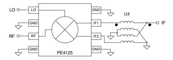
U4 M/A-Com E-Series RF 4:1 Transformer 2.0 – 1000 MHz ETK4-2T
