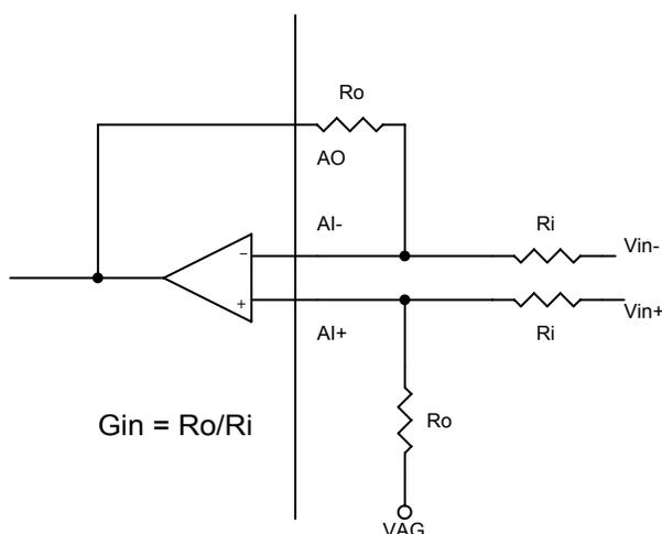
**FIGURE 7.3: INPUT OPERATIONAL AMPLIFIER GAIN – DIFFERENTIAL INPUT**
