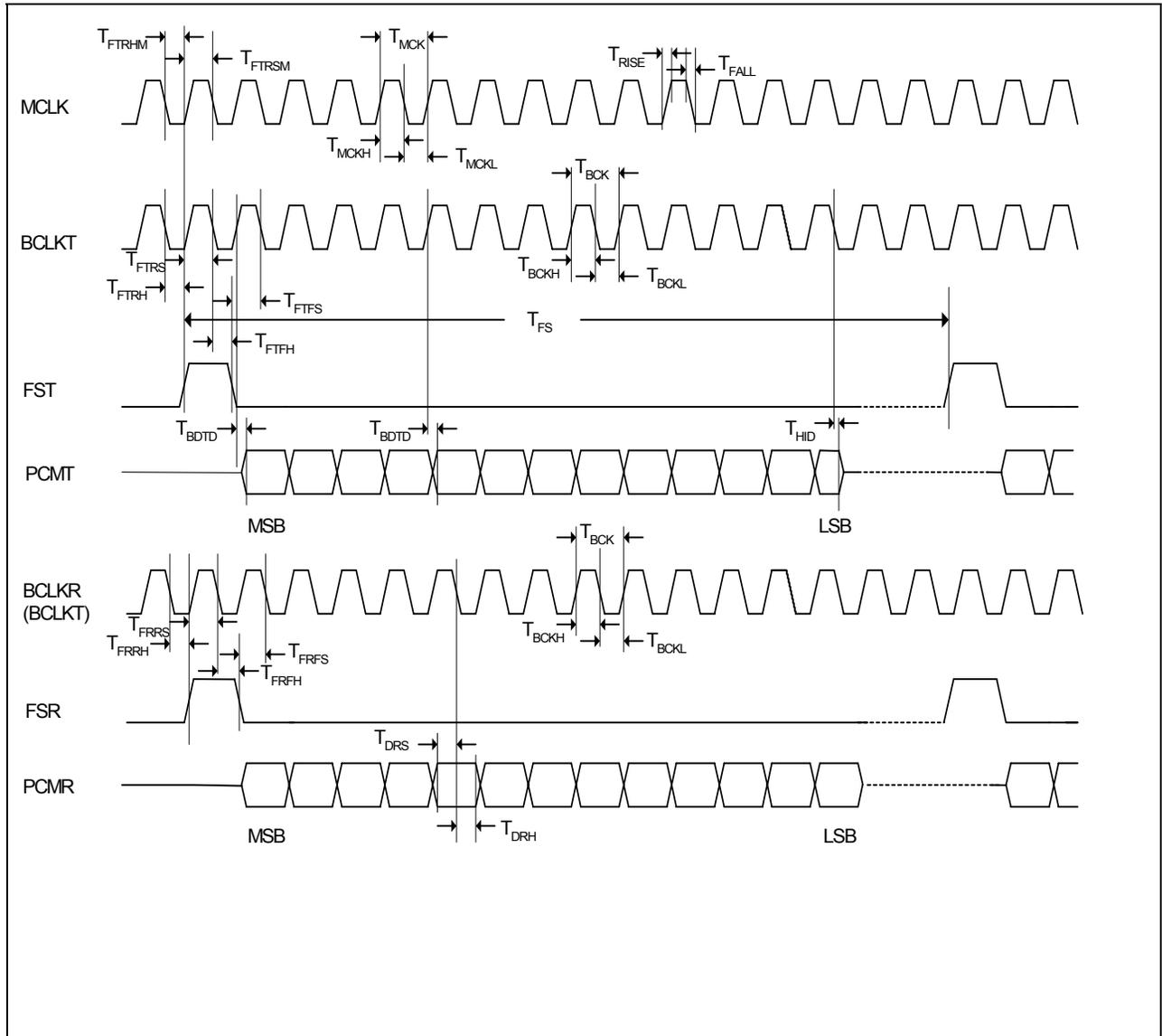
FIGURE 8.2: SHORT FRAME SYNC PCM TIMING
