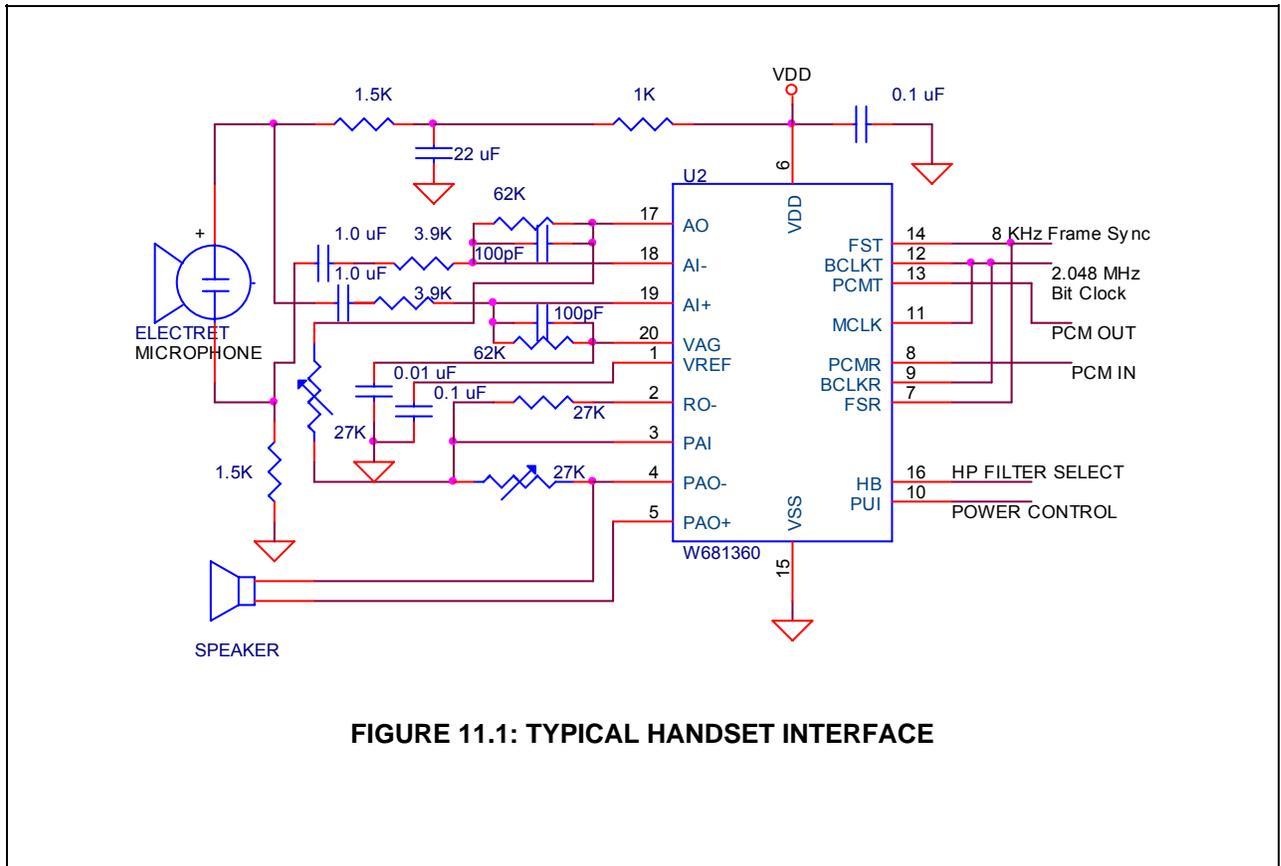
FIGURE 11.1: TYPICAL HANDSET INTERFACE
