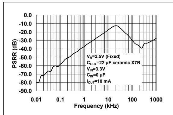
**FIGURE 2-24:** Power Supply Ripple Rejection (PSRR) vs. Frequency.
