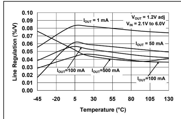
**FIGURE 2-4:** Line Regulation vs. Temperature (Adjustable Version).
