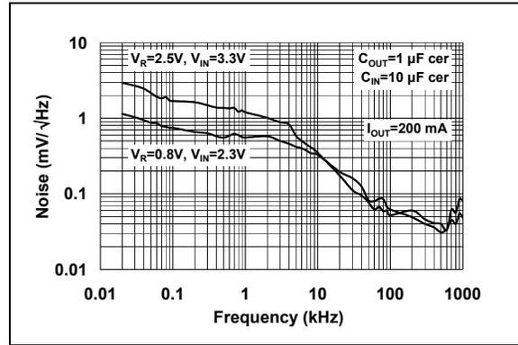
**FIGURE 2-22:** Output Noise Voltage Density vs. Frequency.
