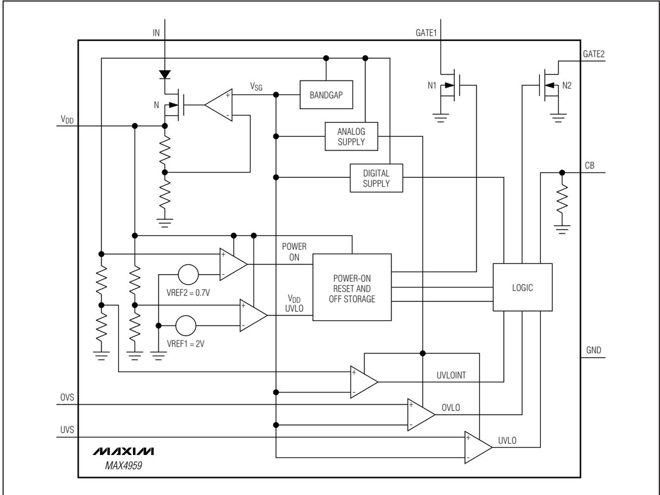
no blanking time for OVP, but the debounce time applies once the IN voltage falls below  $V_{OVLO}$  but above  $V_{UVLO}$ . When the voltage at IN is higher than  $V_{OVLO}$ , the CB pin does not control P1.
