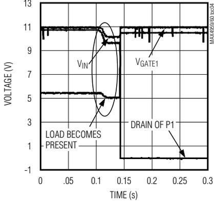
**BATTERY SWITCHOVER WITH ADAPTER-PLUGGED RESPONSE**
