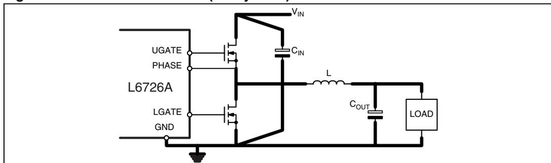
The input capacitance ( $C_{IN}$ ), or at least a portion of the total capacitance needed, has to be placed close to the power section in order to eliminate the stray inductance generated by the copper traces. Low ESR and ESL capacitors are preferred, MLCC are suggested to be connected near the HS drain.
