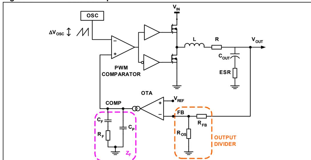
The converter transfer function is the small signal transfer function between the voltage at the output node of the EA (COMP) and  $V_{OUT}$ . This function has a double pole (complex conjugate) at frequency  $F_{LC}$  depending on the L- $C_{OUT}$  resonance and a zero at  $F_{ESR}$
