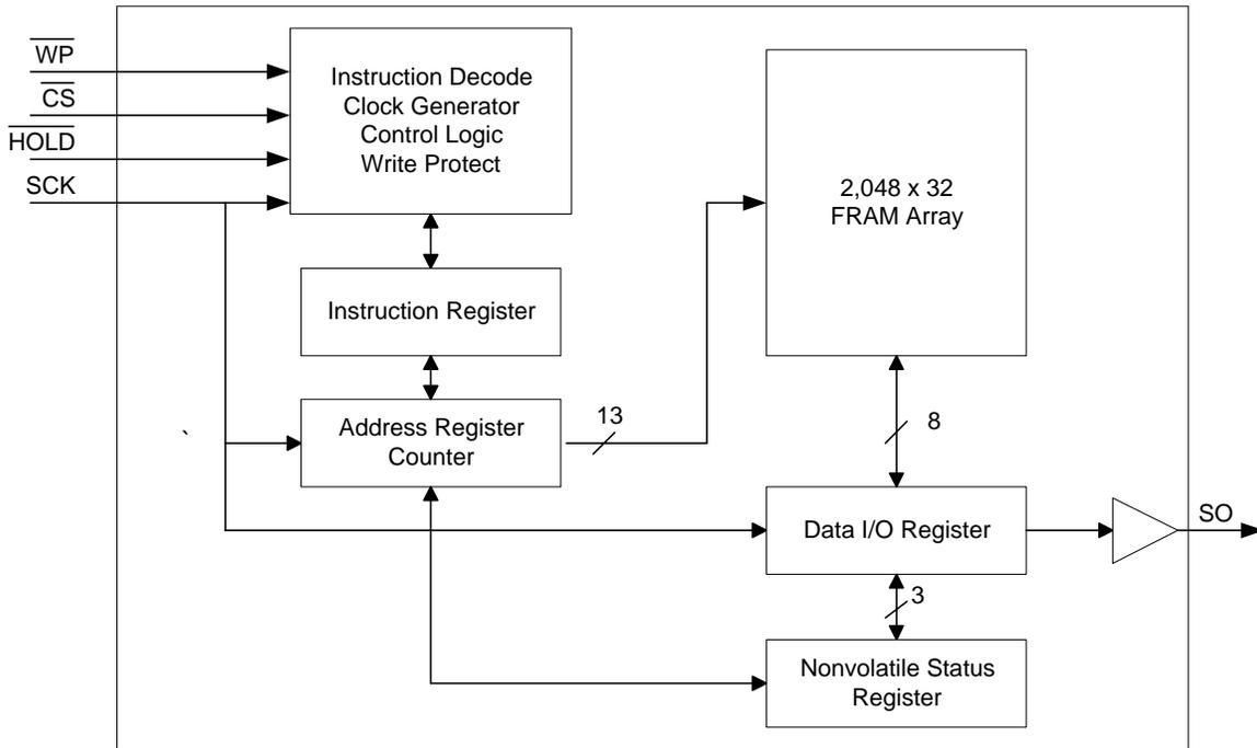
Figure 1. Block Diagram
