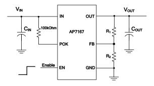
The output voltage is calculated by:
