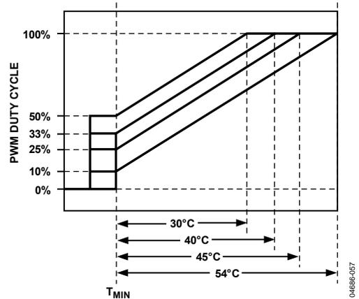
Figure 60. Increasing PWM<sub>MIN</sub> Changes Effective T<sub>RANGE</sub>
