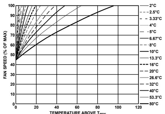
Figure 62.  $T_{RANGE}$  and % Fan Speed Slopes with  $PWM_{MIN} = 20\%$
