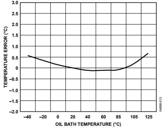
Figure 13. Remote Temperature Error vs. Temperature
