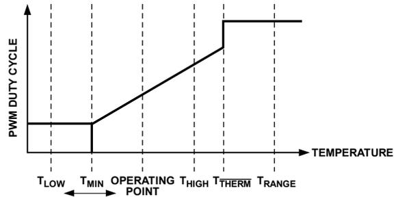
Figure 68. Dynamic  $T_{MIN}$  Control Loop
