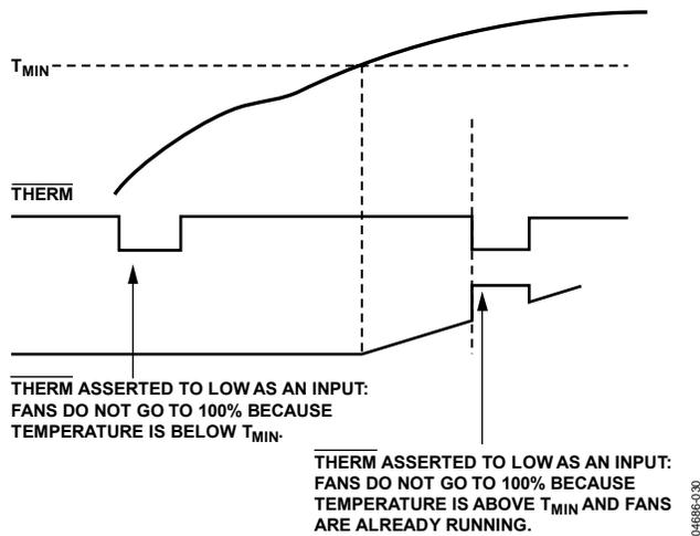
Figure 33. Asserting  $\overline{THERM}$  Low as an Input in Automatic Fan Speed Control Mode
