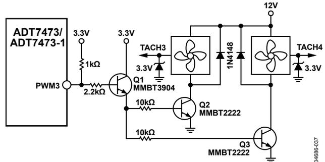
Figure 40. Interfacing Two Fans in Parallel to the PWM3 Output Using Low Cost NPN Transistors
