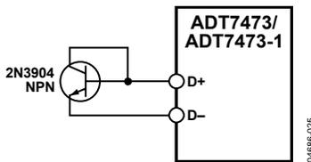
Figure 27. Measuring Temperature Using an NPN Transistor
