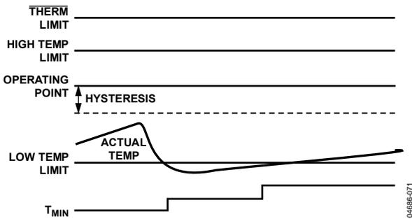
Figure 74. Increasing  $T_{\text{MIN}}$  for Quieter Operation
