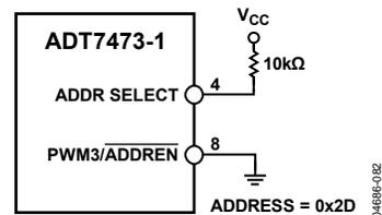
Figure 17. SMBus Address = 0x2D (Pin 4 = 1)
