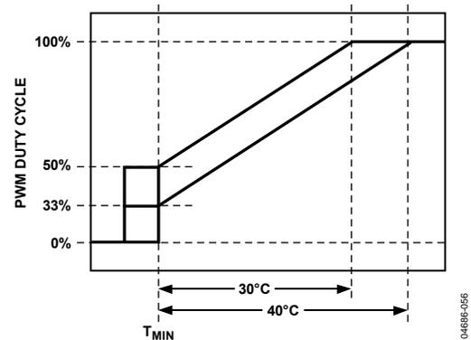
Figure 59. Adjusting PWM<sub>MIN</sub> Affects T<sub>RANGE</sub>
