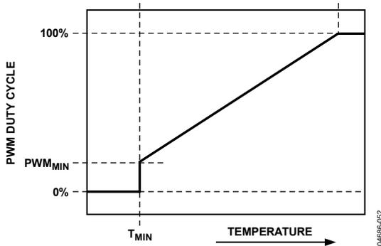
Figure 55. PWM<sub>MIN</sub> Determines Minimum PWM Duty Cycle
