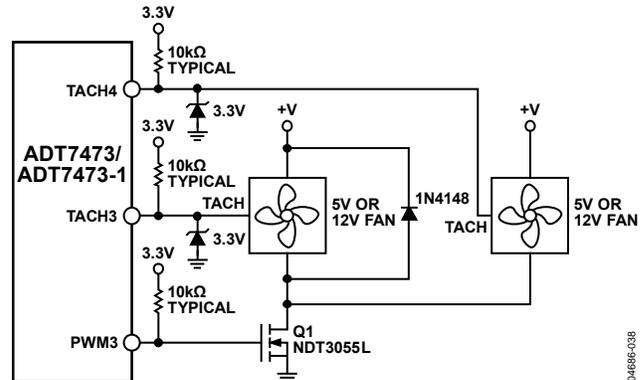
Figure 41. Interfacing Two Fans in Parallel to the PWM3 Output Using a Single N-Channel MOSFET
