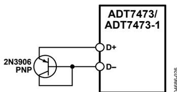
Figure 28. Measuring Temperature Using a PNP Transistor
