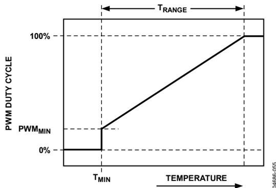
Figure 58. T<sub>RANGE</sub> Parameter Affects Cooling Slope
