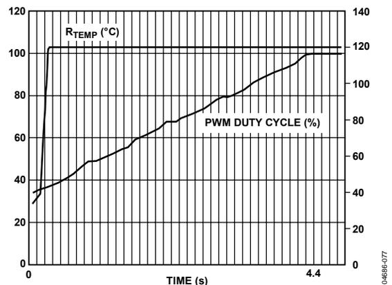
Figure 80. Enhanced Acoustics Mode with Ramp Rate = 8
