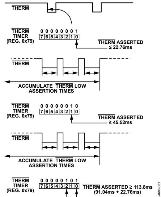
Figure 34. Understanding the  $\overline{THERM}$  Timer
