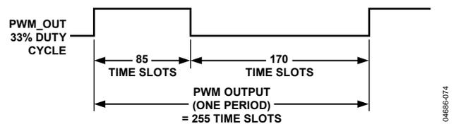
Figure 77. 33% PWM Duty Cycle Represented in Time Slots
