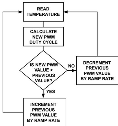
Figure 78. Enhanced Acoustics Algorithm
