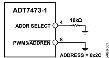
Figure 16. SMBus Address = 0x2C (Pin 4 = 0)
