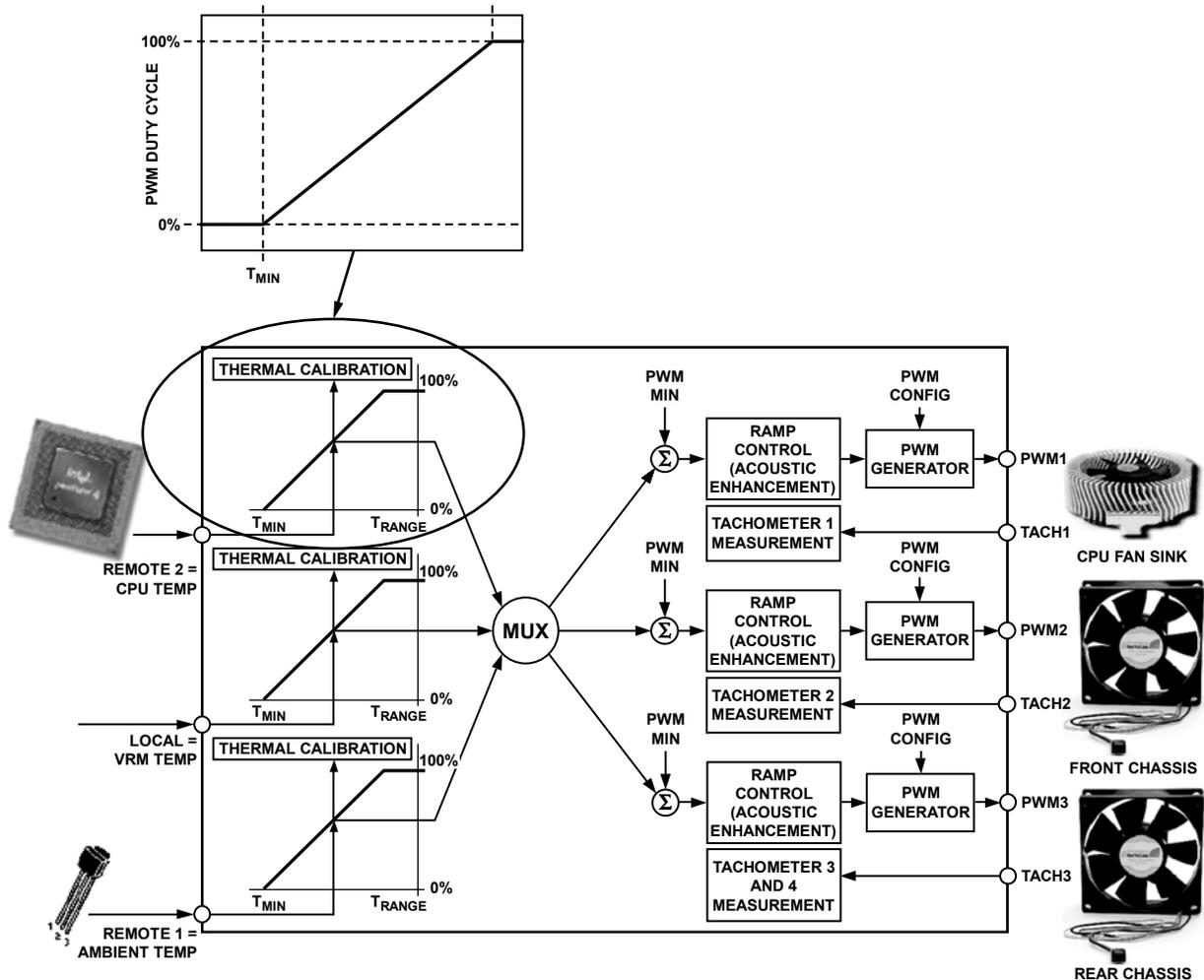
Figure 54. Understanding the T<sub>MIN</sub> Parameter
