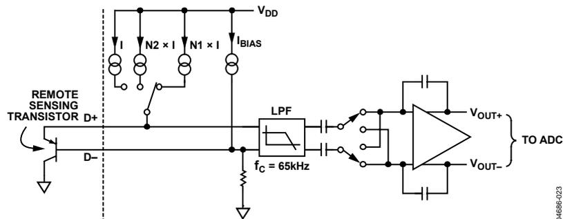
Figure 26. Signal Conditioning for Remote Diode Temperature Sensors
