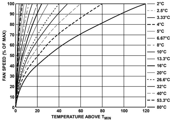
Figure 61.  $T_{RANGE}$  vs. Actual Fan Speed Profile
