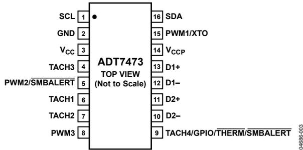
Figure 3. ADT7473 Pin Configuration
