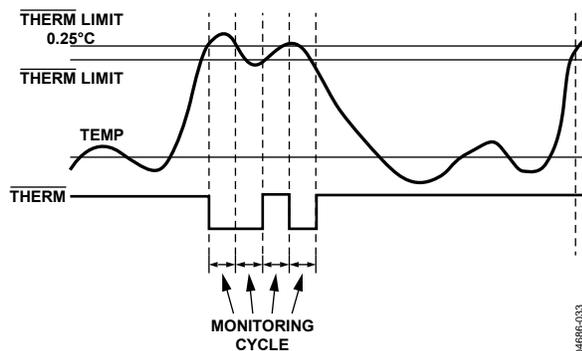
Figure 36. Asserting  $\overline{\text{THERM}}$  as an Output, Based on Tripping  $\overline{\text{THERM}}$  Limits
