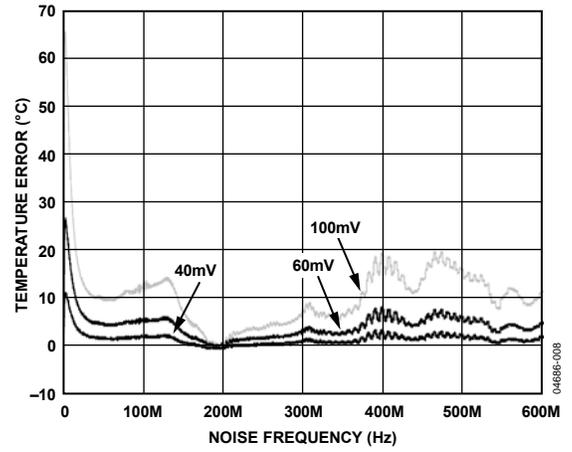
Figure 8. Remote Temperature Error vs. Common-Mode Noise Frequency
