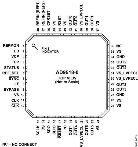
Figure 4. Pin Configuration
