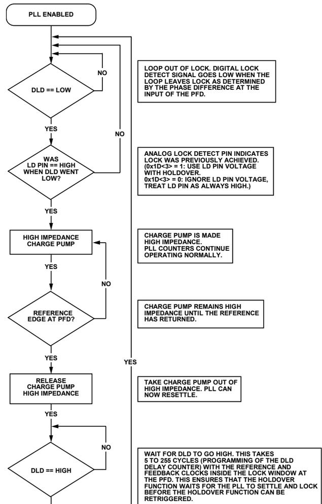
Figure 36. Flow Chart of Automatic/Internal Holdover Mode
