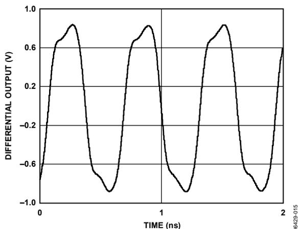
Figure 15. LVPECL Output (Differential) @ 1600 MHz
