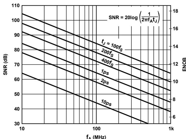
Figure 50. SNR and ENOB vs. Analog Input Frequency
