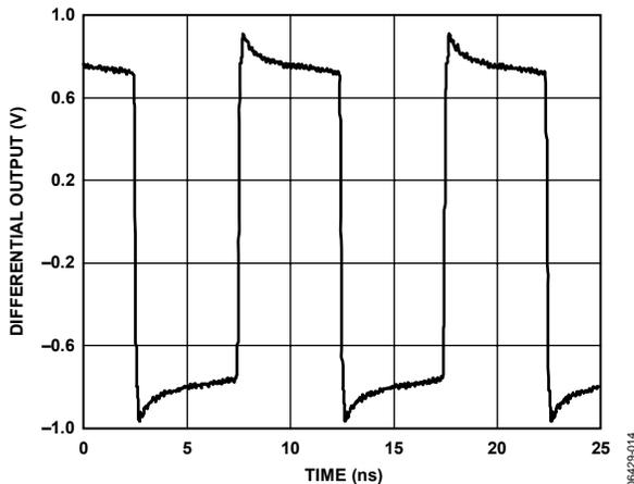
Figure 14. LVPECL Output (Differential) @ 100 MHz
