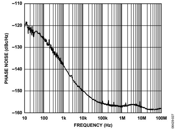
Figure 21. Phase Noise (Additive) LVPECL @ 200 MHz, Divide-by-5
