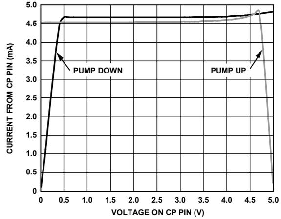
Figure 8. Charge Pump Characteristics @  $V_{CP} = 5.0 V$
