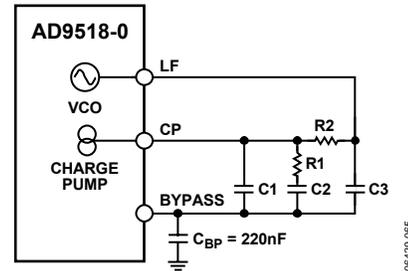
Figure 31. Example of External Loop Filter for PLL
