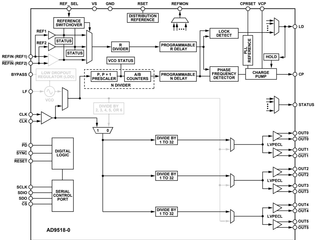
Figure 29. Clock Distribution or External VCO < 1600 MHz
