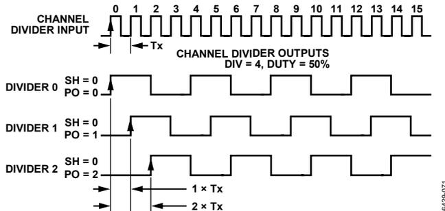
Figure 38. Effect of Coarse Phase Offset (or Delay)
