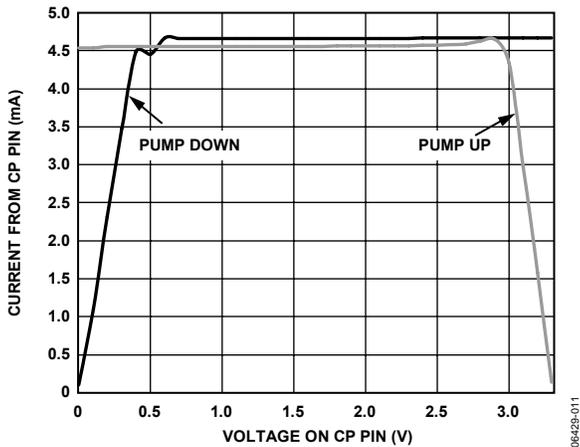
Figure 7. Charge Pump Characteristics @  $V_{CP} = 3.3 V$
