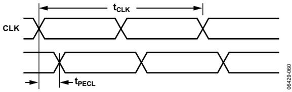
Figure 2. CLK/ $\overline{\text{CLK}}$  to Clock Output Timing, DIV = 1
