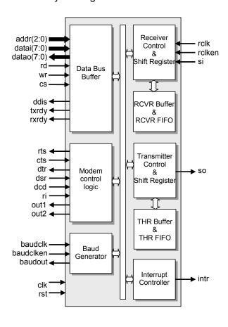
**Baud Generator** - The D16550 contains a programmable 16 bit baud generator that divides clock input by a divisor in the range between 1 and (2<sup>16</sup>–1). The output frequency of the baud generator is 16× the baud rate. The formula for the divisor is:
