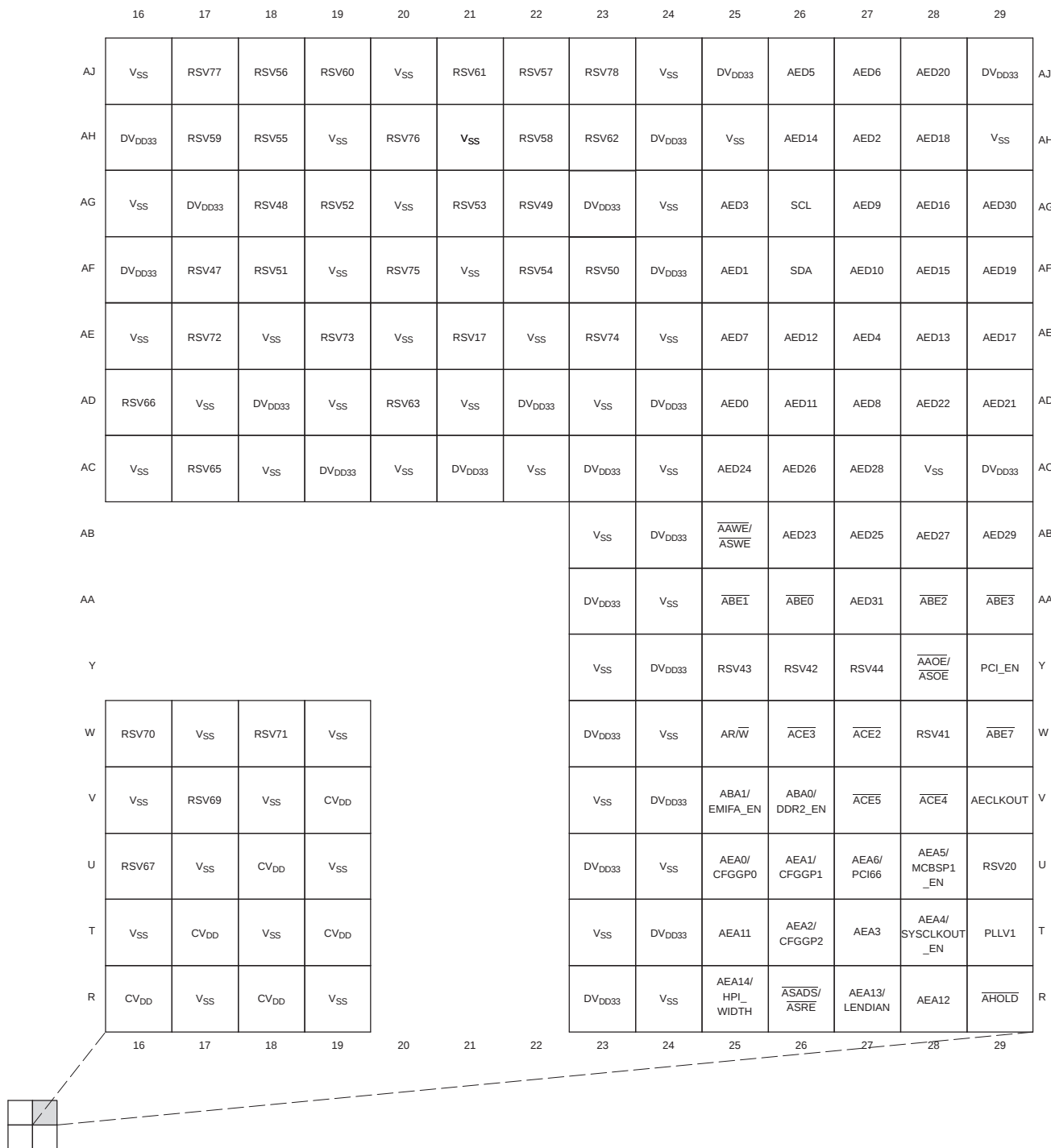
Figure 2-3. C6454 Pin Map (Bottom View) [Quadrant B]
