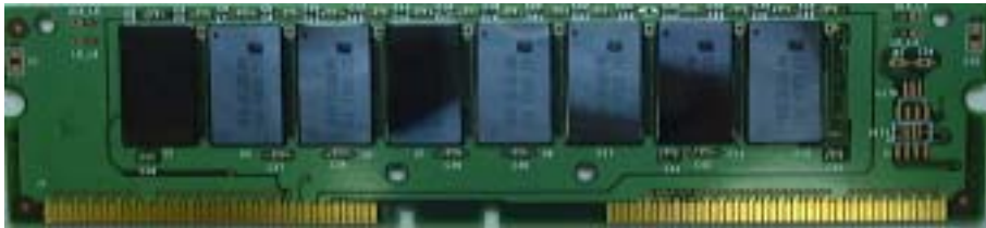
Figure 1: RIMM Module shown with heat spreader removed
