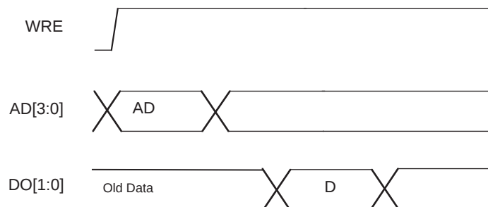
Figure 3-7. Slice Single /Dual Port Read Cycle Timing
