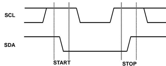
FIGURE 10. I<sup>2</sup>C START AND STOP BITS
