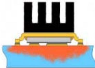
⑨ Mounted to a PCB with small clip heatsink (still air)
