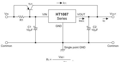
$$R_1 = \frac{V_{BE1}}{I_{REG} - \frac{I_{C1}}{(1+\beta)}}$$
