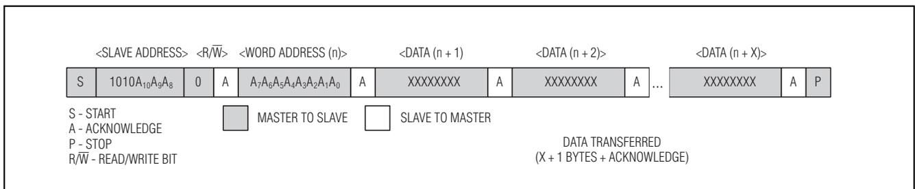
Figure 5. Data Write—DS32B35 FRAM Slave Receiver Mode
