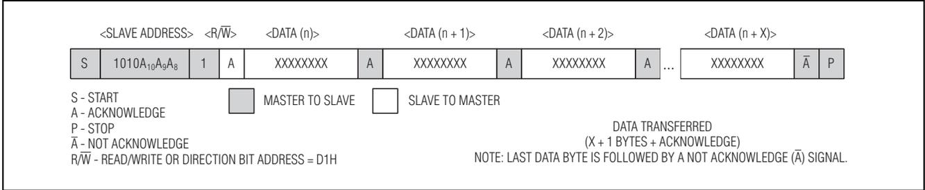
Figure 6. Data Read—DS32B35 FRAM Slave Transmitter Mode
