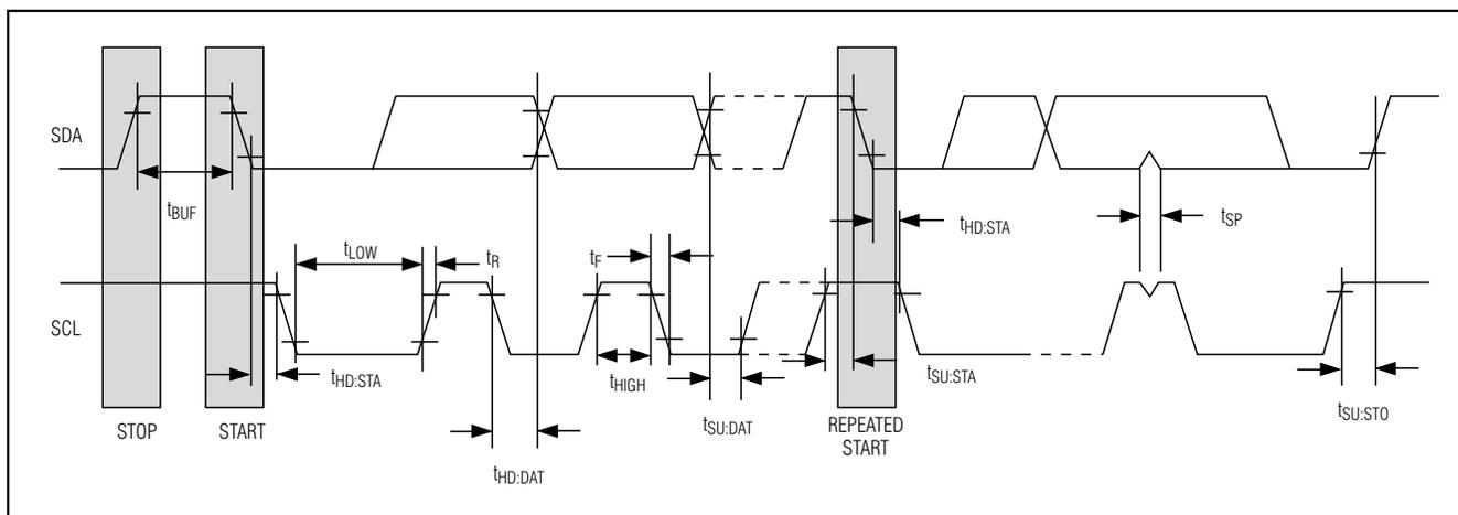
Figure 1. Data Transfer on I<sup>2</sup>C Serial Bus
