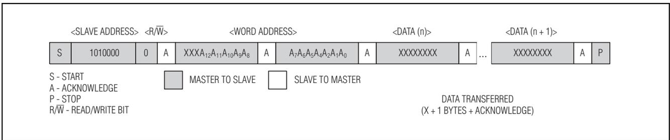
Figure 7. Data Write—DS32C35 FRAM Slave Receiver Mode
