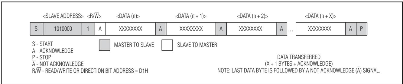
Figure 8. Data Read—DS32C35 FRAM Slave Transmitter Mode
